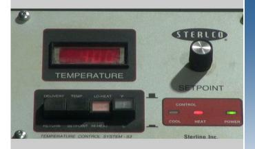
We've reached the maximum rated temperature. We will turn off the heating circuit and let the unit return to room temperature before shutting the system down.
