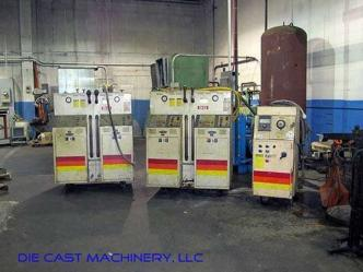
**Description:** Used, Sterlco Model M2B 9026-J0 48 kW (24 kW per zone) Dual (two) Zone Portable Hot Oil Process Heater Temperature Control Unit For Sale, Features include: Sterlco M2B Microprocessor Temperature Control System, Alarms for low fluid pressure, pump rotation, over temperature, Set points for Process, High Alarm, Low Alarm, Displays for Process Temperature, Return Temperature and Temperature Difference, , , M2B Sterling Stearl-Tronic Controls, Second Hand, DCM-2661
