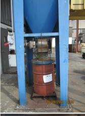
U.S. Filter/ BCP JPSM-2D 4 Dust Collector Serial #2994
